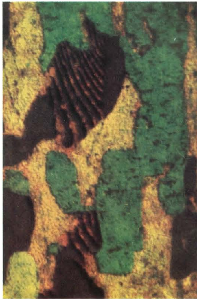
Fig. 9. \text{FeCl}_3 hydrolysate, crystals of higher order, twinned, reflected light, green and yellow of first order, light vector parallel to the short side ( \times 405 ).
