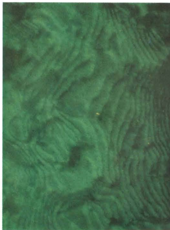
Fig. 10. The same as Fig. 9, light vector parallel to the long side. The isotropic, brown reflecting, mostly striated parts are probably transformation products of crystals of higher order.
